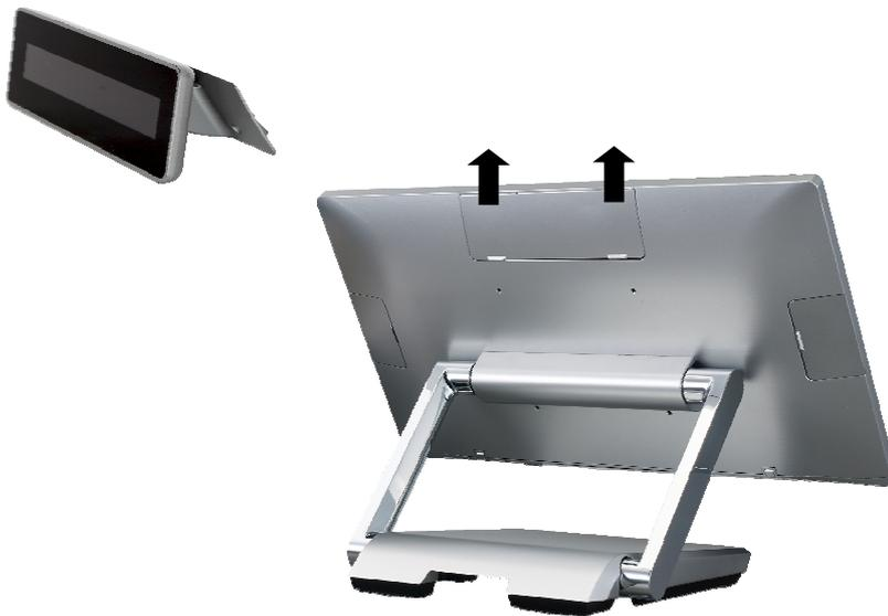
5. Install the two screws that attached the customer display to panel head.
