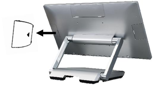
2. plug in ID device (USB) and fix it via 1 x M3 screw
